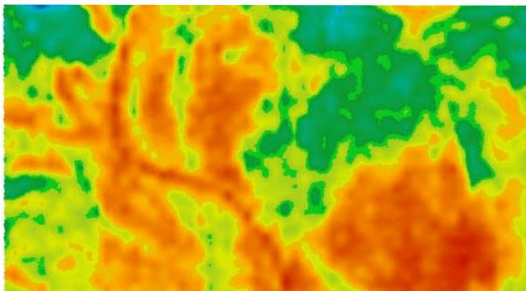
Figure 2.6.10. Slope map to identify possible hollows or ridges
