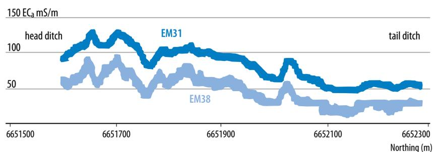
What is also apparent in Figure 2.6.3b is a small band of low  $EC_a$  (that is, <100 mS/m) which lies perpendicular to the eastern storage wall at an approximate Northing of 6651750 (sample site 19). This lower band of soil  $EC_a$  is more evident in Figure 2.6.4 for both EM instruments (that is, Northing 6651750).
