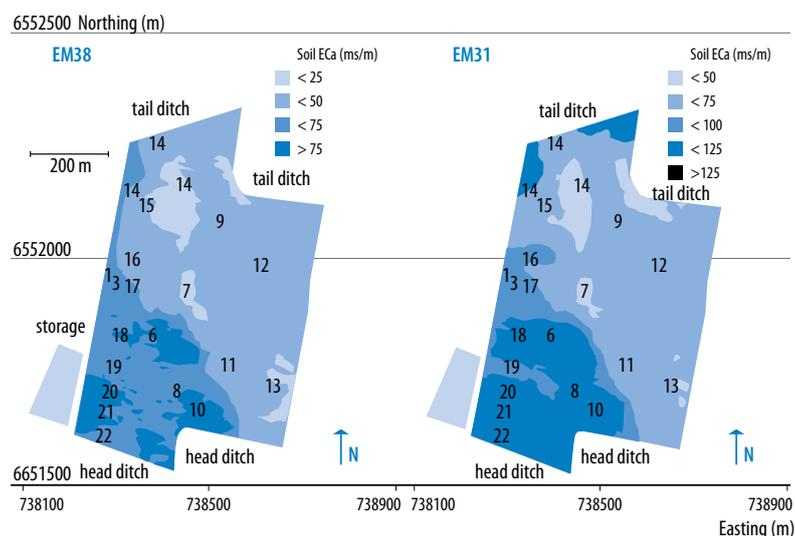
It is also evident that a sharp drop in  $EC_a$  occurs approximately halfway between the head and tail ditch. This drop in soil  $EC_a$  is shown more clearly in Figure 2.6.4, along transect 3.
